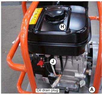
The oil drain plug is located at the bottom of the engine block. Place a pan under the drain and remove the plug. Drain the oil and replace the plug. Using a long neck funnel, fill the engine with 0.6 quarts (0.6 liters) of oil. When full, the oil level should be at the high level mark on the dipstick (A) or to the top of the threads on the engine fill hole. The engine is equipped with an oil alert system that will stop the engine if the oil level is low.
