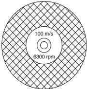
Ensure the blade is not cracked or damaged in any other way.
