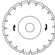
Always use a sharp diamond blade. Sharpen the blade by cutting in a soft material such as sandstone or brick.
