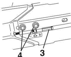
Screw in the tension screw (3) so that the square nut aligns with the arrow on the belt guard. Shake the head to ensure the spring can tension the belt. This automatically adjusts the belt to the correct tension. Tighten both bolts (4) using the combination spanner. **NOTE!** When a belt is fitted the belt tension must be readjusted after the first two tanks of fuel have been used.
