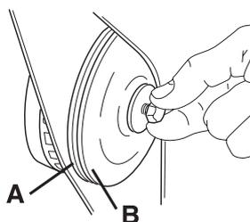
The shaft can be locked using a screwdriver, steel pin or the like. This is slid in as far as possible. The blade is tightened clockwise.
