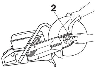
Position the belt guard and secure the cutting head together with the belt guard. Tighten both bolts (4) by hand.
