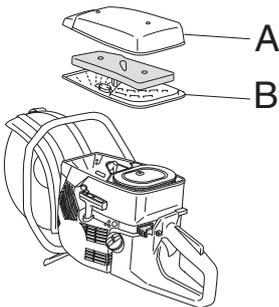
Remove the foam plastic filter. Wash the filter well in tepid soapy water. After cleaning, rinse the filter well in clean water. Squeeze out and allow the filter to dry. **NOTE!** High pressure compressed air can damage the foam.
