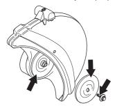
Do not use warped, notched, indented or dirty flange washers. Do not use different dimensions of flange washers.
