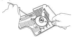
Secure the starter cord around the cord pulley as illustrated. Tighten the fastening well and ensure that the free end is as short as possible. Secure the end of the starter cord in the starter handle.
