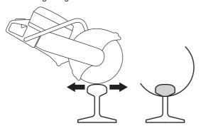
When you have cut through the head (A), you continue cutting the rib (B) and foot (C).
