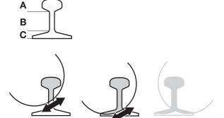
If the cut cannot be completed from one side, the power cutter must be turned around.
