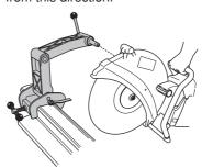
NOTICE! The rail fixture must be first fitted to the rail before the power cutter is fitted to the rail fixture. This is done to guarantee that the fixture is attached at right angles to the rail.
