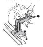
Guide the cutting blade down towards the rail and check that the cutting blade is centred in the cut. If necessary, adjust the movable bushing so that the blade ends up centred in the middle of the cut.
