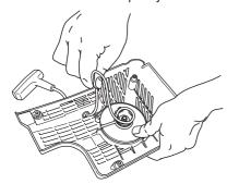
Now pull the starter handle and in doing so tension the spring. Repeat the procedure once more, but this time with four turns.
