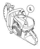
NOTICE! A too lean adjusted low speed needle (the Lneedle closed too much) results in starting difficulties.
