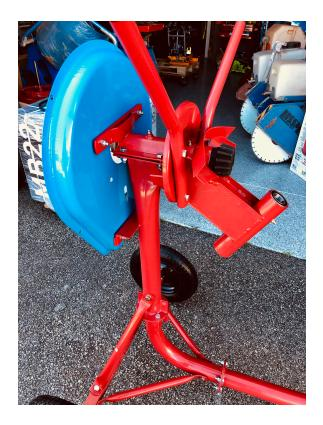
bowl over as if tipping cement out gives clearest view of pinion. If pinion and gearwheel mesh is not adjusted correctly, the pinion wheel will wear prematurely. We stock and sell these because customers do not adjust them correctly! Once adjustment is made, it may be easier to remove bowl again and grease nipple closest to pinion - it is hard to get behind bowl.
