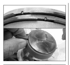
Assemble the cylinder Check that the opening on the piston rings align with the guide pin.
