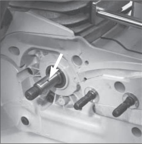
**Model 1250 – Crankcase lubrication hole**
