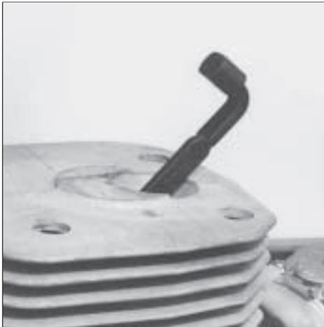
Fit piston stop No. 502 54 15-01 in the spark plug hole.
