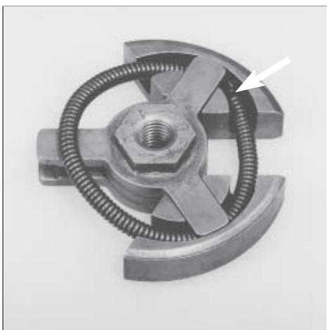
Fit together the centrifugal clutch.
