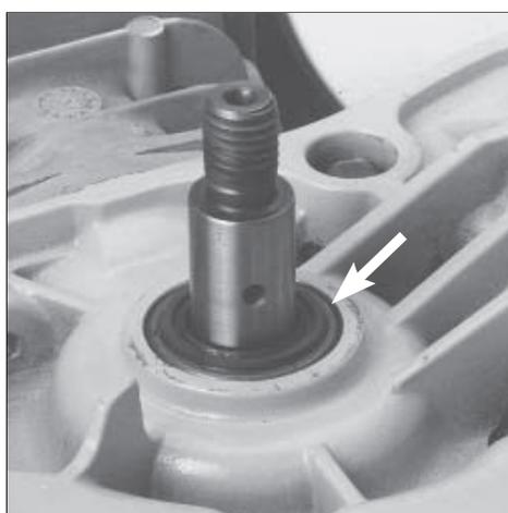
Dismantle the seal with an extractor 504 91 40-01.
