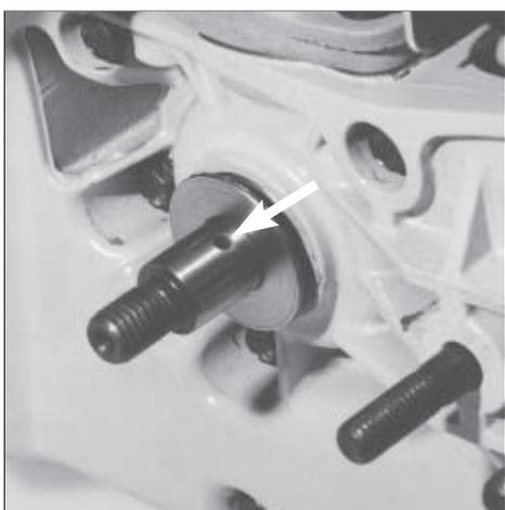
Check that the lubrication hole in the crankshaft is not blocked.
