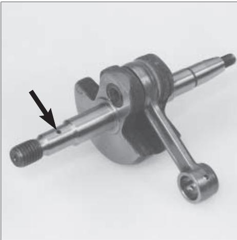
Blow clean the channel for the automatic lubrication of the clutch drum's bearing.
