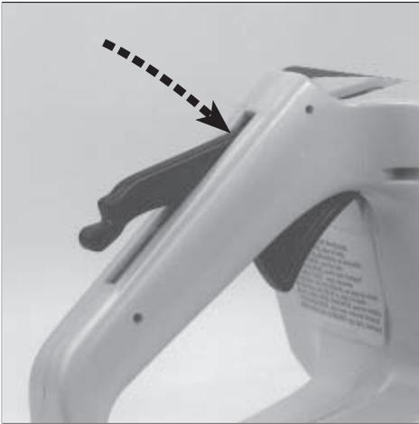
Press the safety catches forwards/downwards and lift them up at the back edge.
