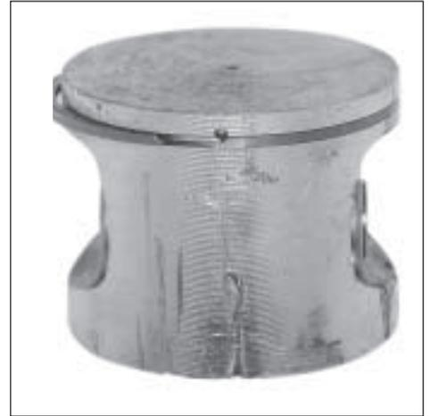
*Irregular grooves on the piston's inlet side caused by a broken bearing cage.*
