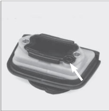
Inspect the spacing piece and intake pipe for signs of cracking and other damage. Check that the impulse channel is open.
