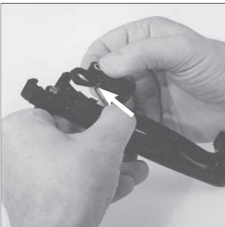
Hook in the spring in the hole in the throttle control and move it to the correct position opposite the screw hole.
