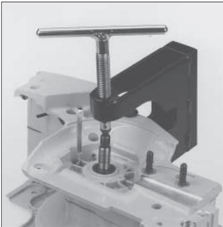
Separate and assemble the crankcase halves in the same way as described for mod. 650, 700.
