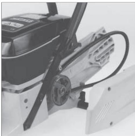
Fit the drive belt and the rear belt cover in the same way as for mod. 650, 700.
