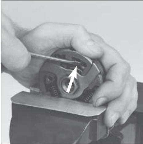
Clean and inspect the clutch parts for damage and wear.
