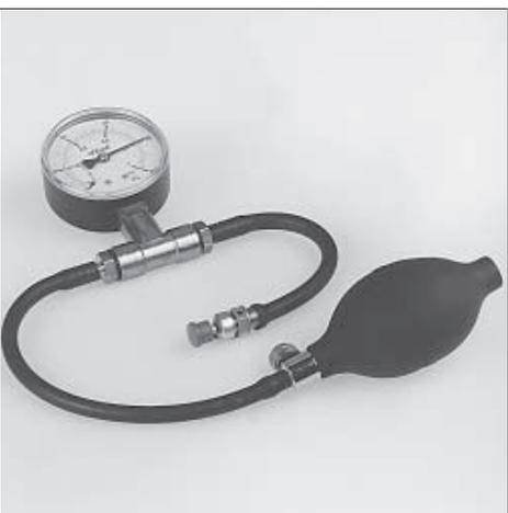
Check that the valve is tight with pressure gauge 502 50 38-01.
