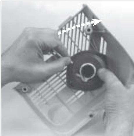
Wind the pulley 7 turns *clockwise*.
