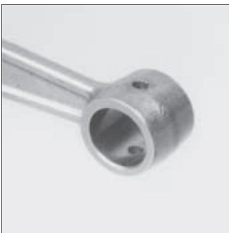
Check the connecting rod's small end.
