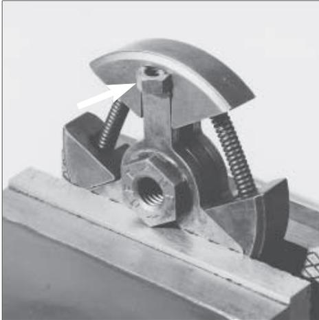
Place an object which is approx. 5.5 mm (0.22") thick between the clutch shoe and the spoke.
