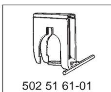
Use the same tool as above and press out the crankshaft from the crankcase half.
