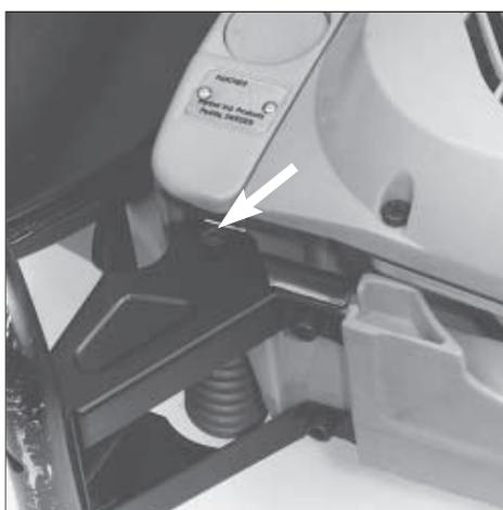
Separate crankcase and tank unit and remove the screw which holds the vibration damper.
