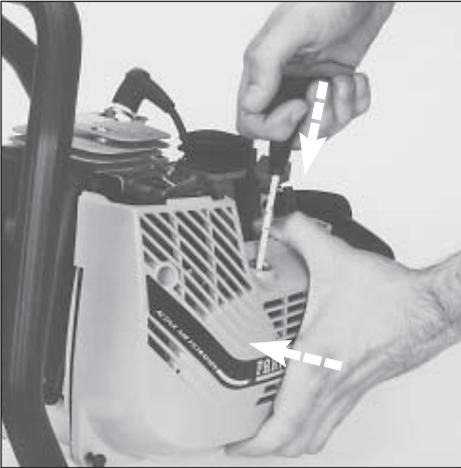
Fit the starter unit and other parts in the reverse order to dismantling.
