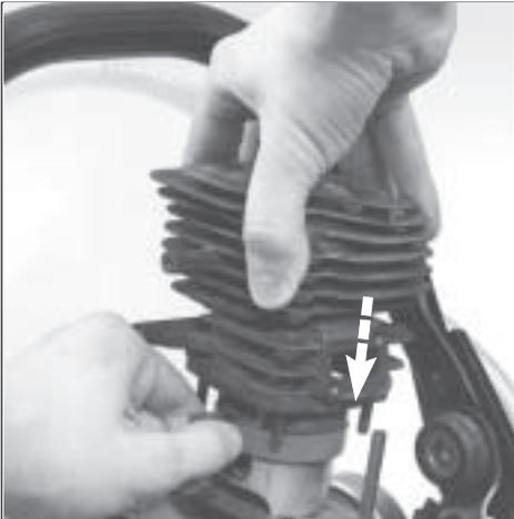
Lubricate the cylinder bore with a few drops of oil and push down the cylinder over the piston.
