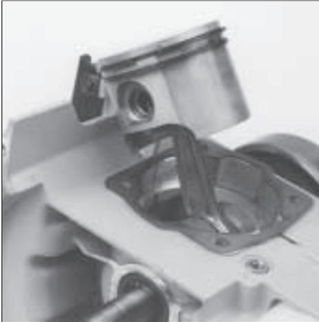
Fit a new cylinder base gasket.
