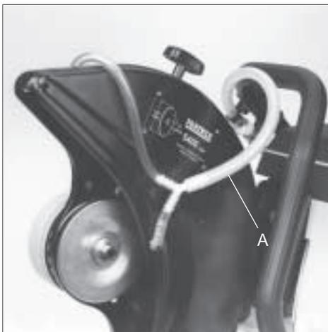
Remove hose (A) if the water accessory has been installed.
