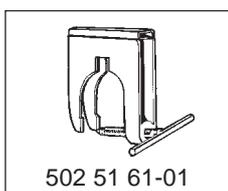
Separate the crankcase halves by means of tool 502 51 61-01.
