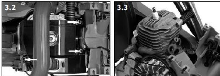
3.2. Dismantle the three screws on the air duct cover.
