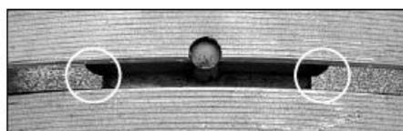
Turn the piston ring with the bevelled edge towards the guide pin.
