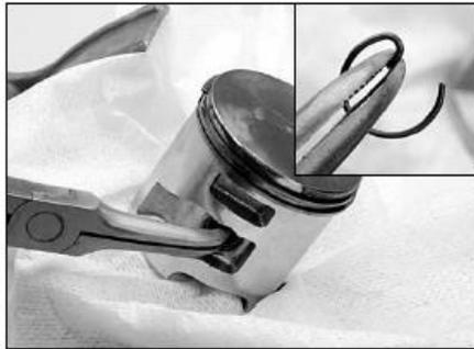
Dismantle the circlips on both sides of the gudgeon pin.
