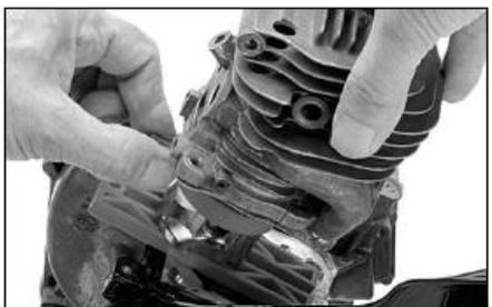
Press down the cylinder over the piston and let the piston ring compressor slide along the piston.
